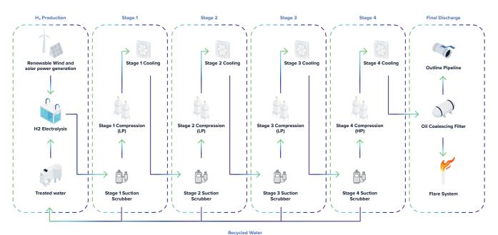
Figure 3.3 Hydrogen Compression Process
