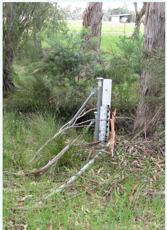
One of the staff gauges, used to measure water height, at Willyung Creek, October 2006.
