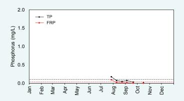
2018 phosphorus concentrations at 6091225. The black dashed line is the Scott River WQIP target for TP, the red is the ANZECC trigger value for lowland rivers for FRP.
