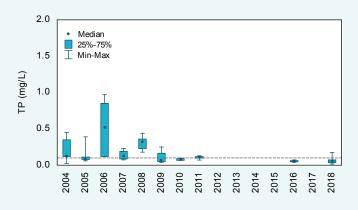
Total phosphorus concentrations, 2004–18 at site 6091225. The dashed line is the Scott River WQIP target for median TP concentrations.
