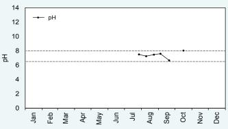
2018 pH levels at 6091225. The dashed lines are the upper and lower ANZECC trigger values for lowland rivers.
