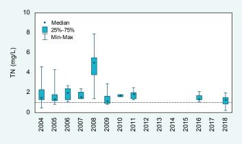
Total nitrogen concentrations, 2004–18 at site 6091225. The dashed line is the Scott River WQIP target for median TN concentrations.
