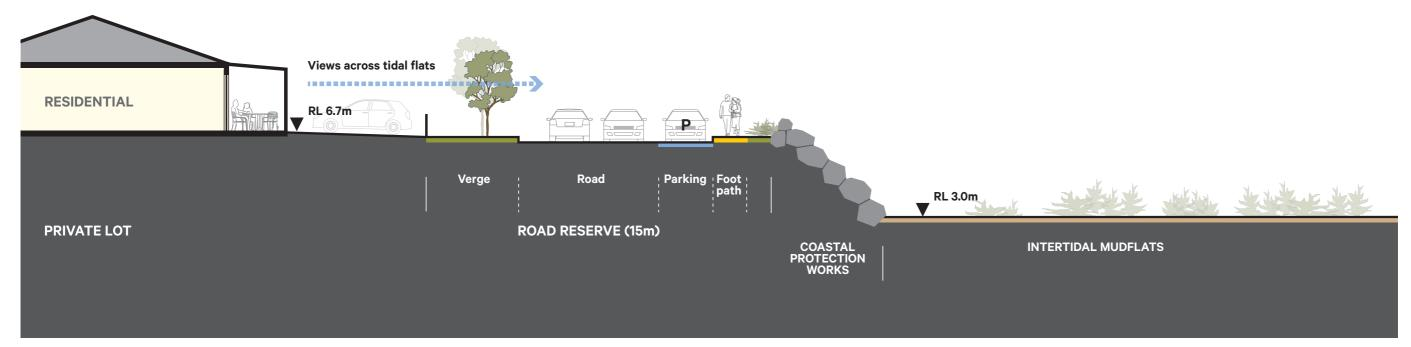
Indicative section showing relationship of road, pedestrian footpath, coastal protection works and level change to mudflats.
