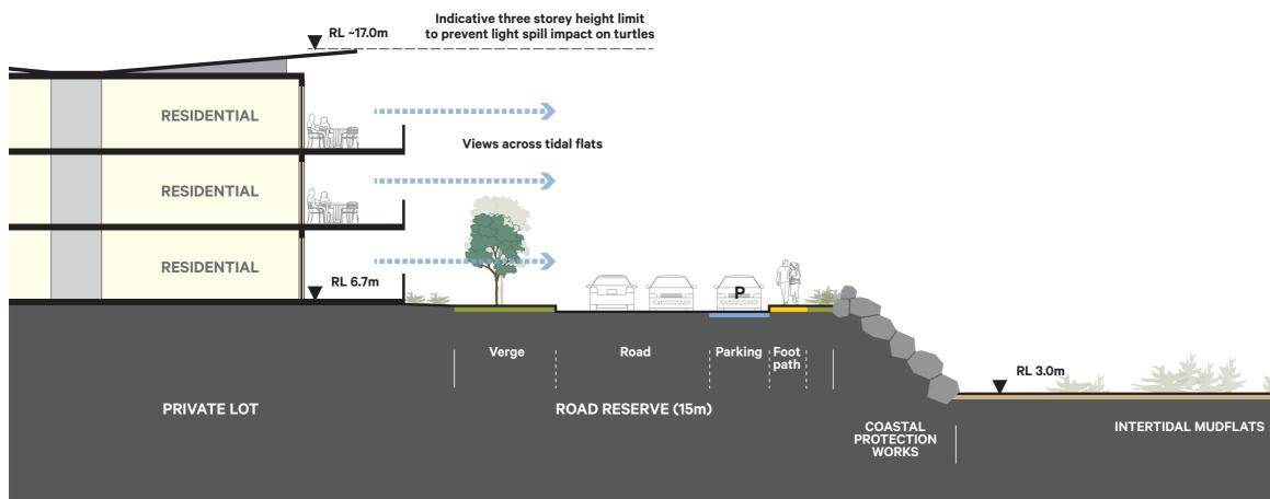
Indicative section showing relationship of road, pedestrian footpath, coastal protection works and level change to mudflats.
