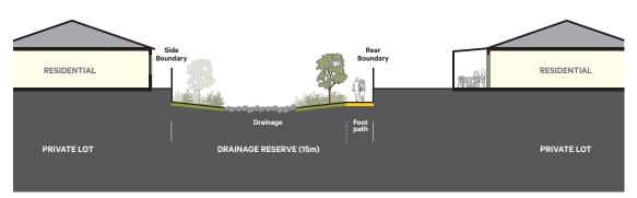
$\label{eq:link} \mbox{Indicative section showing arrangement of drainage link and footpath to proposed dwellings.}$
