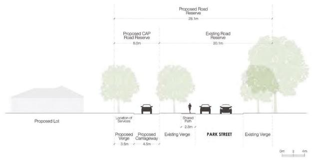
Figure 17: CAP Road Cross-section
